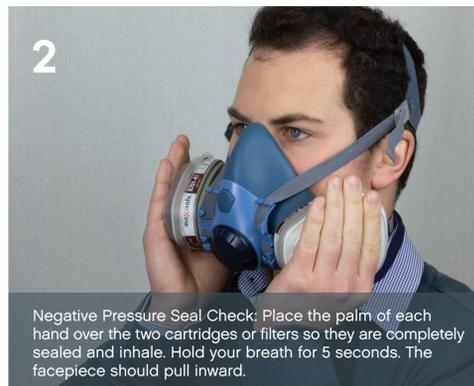
2 Negative Pressure Seal Check: Place the palm of each hand over the two cartridges or filters so they are completely sealed and inhale. Hold your breath for 5 seconds. The facepiece should pull inward.
