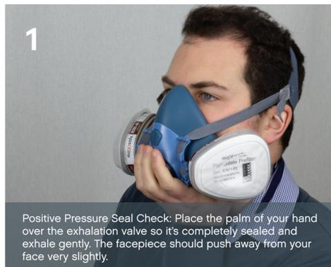
1 Positive Pressure Seal Check: Place the palm of your hand over the exhalation valve so it's completely sealed and exhale gently. The facepiece should push away from your face very slightly.
