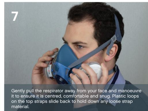
7 Gently pull the respirator away from your face and manoeuvre it to ensure it is centred, comfortable and snug. Plastic loops on the top straps slide back to hold down any loose strap material.
