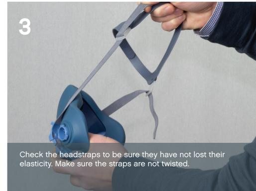
3 Check the headstraps to be sure they have not lost their elasticity. Make sure the straps are not twisted.
